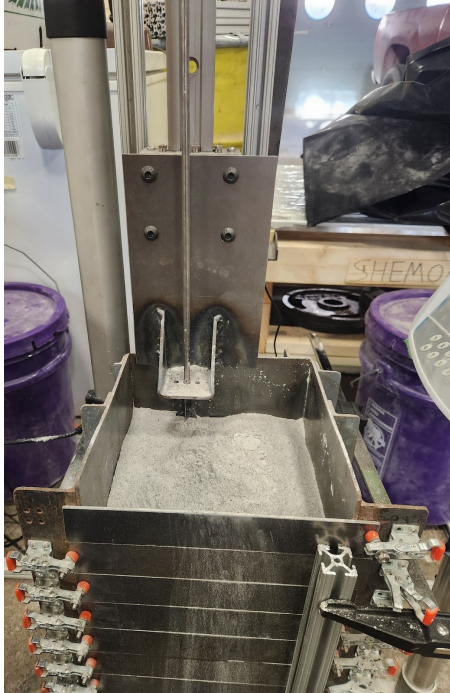
Figure 3: Test box, pin and pressure plate of test setup
